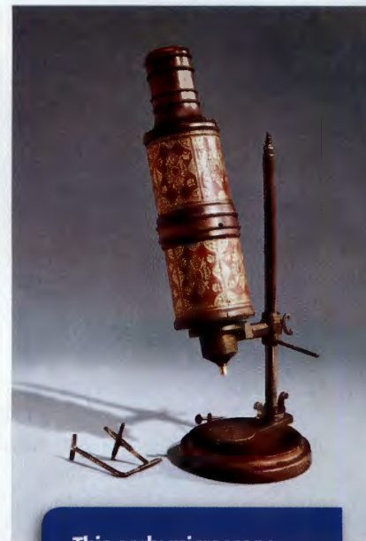
This early microscope was made around 1675. The lens is protected by cardboard and leather and slides up and down.
